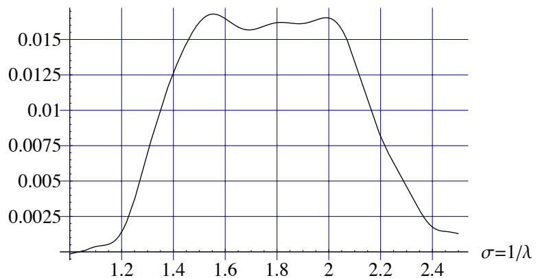
Fig. 9 - Global transmission of the source, optics and detector in the experiment. Notice that the source could nearly be considered as a triple "gaussian" source.
