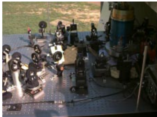
Fig. 12 - Top and side views of the 2-Telescope Breadboard at Meudon Observatory in March 1997.
