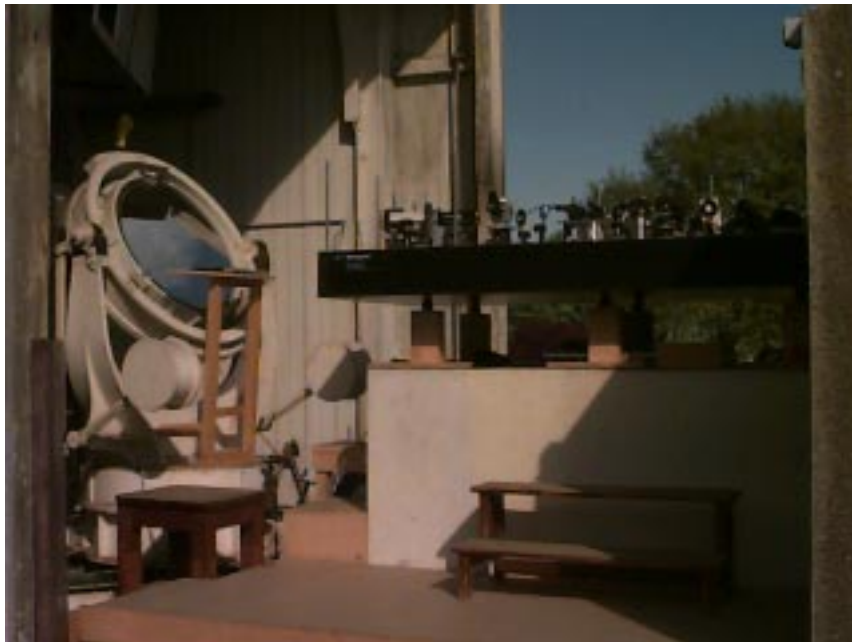
Fig. 11 - The 2-Telescope Breadboard of the Solar Interferometer at the "Grand Sidéostat de Foucault" at Meudon Observatory in March 1997.
